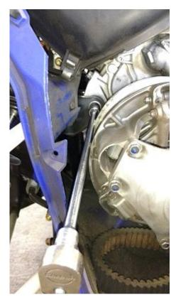
use a 18mm socket with a half drive ratchet on the nut.
