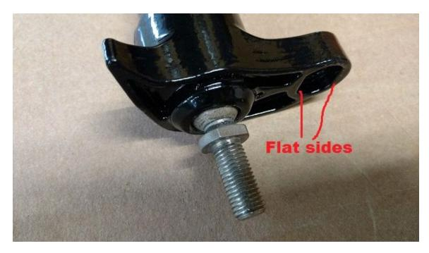
next step is to remove the motor mount nuts, first remove clutch side using a 15mm socket and long extention on the bolt.
