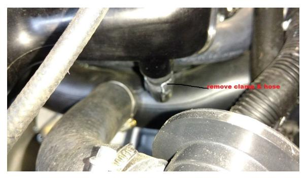
next you can loosen the clamp on the blow off valve shown in the picture below and then pull the hose off and swing it off to the RH side.
