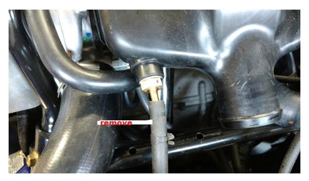
next loosen the three hose clamps on the airbox shown below.
