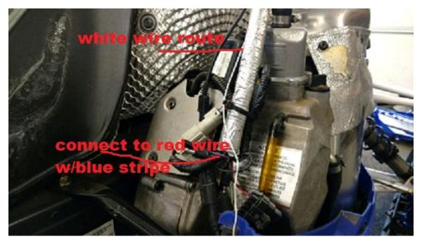
now you may reinstall the sensor/relay plate and then the fuse box.
