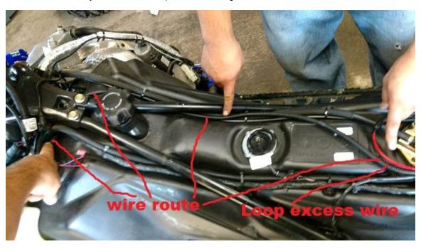
connect white wire using the supplied red connector to the red W/ blue stripped wire from the accessory plug. see picture on next page
