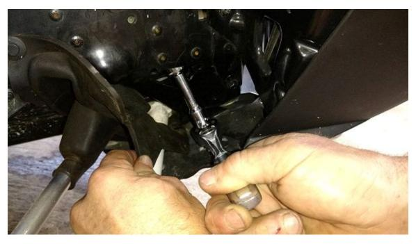
after removing the steering post nut you can pull the post up and out.
