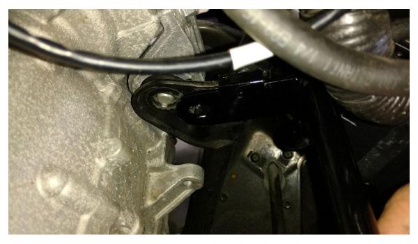
once in place you can push both engine mount bolts back in all the way and put the nuts on but dont tighten them yet. next you can install and tighten the three bolts in the steering motor shown in the picture on the next page.
