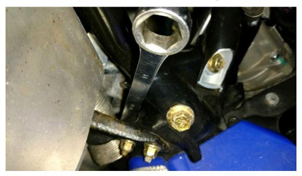
once the Exhaust side nut is off you can slide the bolt out part way so that it is just even with the bracket.
