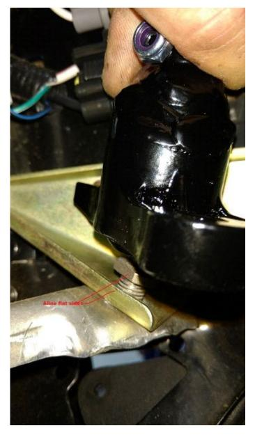
once in position you will have to hold down with some force to keep the stud from rotating while tightening the nut.
