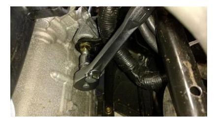
once the nut is off you can slide the bolt part way out - leave it flush with the bracket. now you can remove the other side motor mount nut using a 15mm open end wrench and the same 18mm socket. see picture below for wrench location - kind of tricky!
