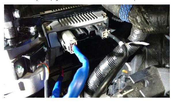
put a ziptie around the steering motor harness and the voltage regulator wires to hold it in place. see picture on next page
