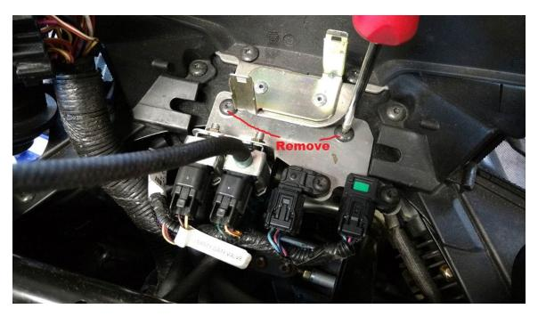
next remove the bolts from the lower side of the handle bar riser. see picture below.
