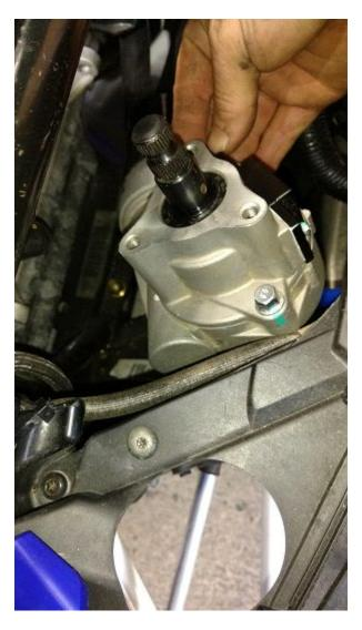
Important: when installing the set screw in the lower end of the steering post you will first want to look in the hole and make sure it is lined up with the groove in the steering motor shaft. once you have it lined up you can put the set screw in and tighten it up with a 5/32 allen wrench. next be sure to tighten the jam nut using a 1/2 inch wrench.
