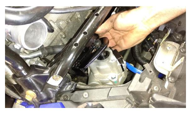
once the mount plate is slid over the upper shaft you can slide the mount plate into position on the engine mounts. see below picture
