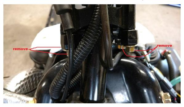
once you have removed all four bolts you can lay the bars back onto the gas tank.
