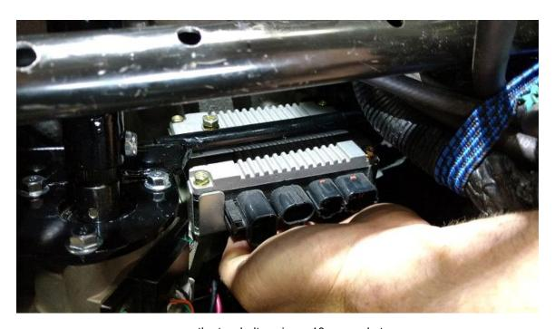
snug the two bolts using a 10mm socket.
