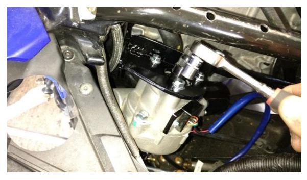
now you can go back and tighten the two engine mount bolts.
