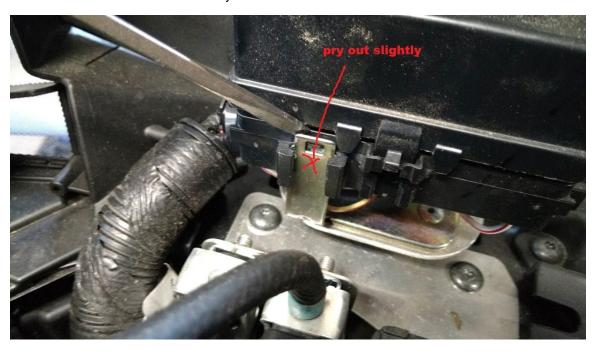
next remove the screws from the sensor/relay mounting plate pictured next using a T25 torx driver. also swing this plate to the RH side out of the way.
