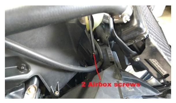
once the lower airbox screws are removed you can loosen the three intake clamps and then prepare to pull the airbox out. you will need to unplug the sensor and pull the hoses and tube from the airbox but the tube will need to be pulled out as you are removeing the airbox.
