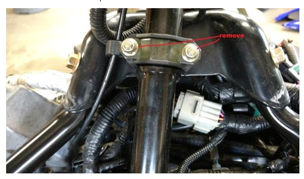
next step is to remove the steering rod from the lower end of the steering post using a 17mm socket. see picture on next page
