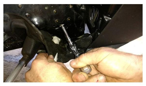
Once you have removed the nut you can pull the steering post out.
