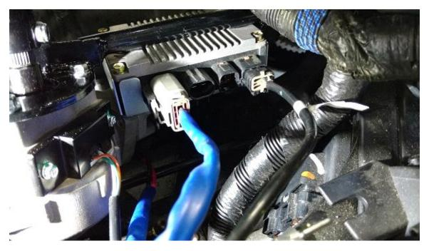
ziptie the wires to the voltage regulator wires shown in the picture on the next page.
