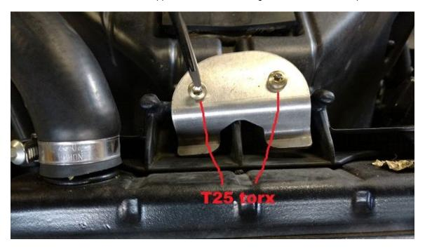
next you will have to pull up on the top of the radiator so you can get to the front airbox screws.
