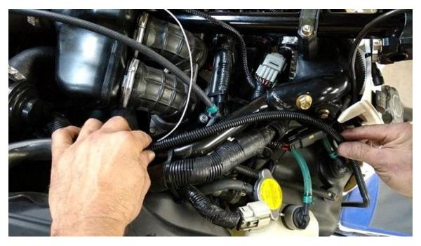
the white wire will branch off towards the clutch cover where you will see a single orange wire in which you will use the supplied red connector to connect to it. see picture on next page
