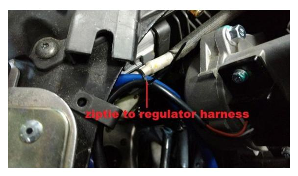
Next plug in the power supply wire harness and run it alone with the snowmobiles main wire harness up the clutch side all the way to the top. see picture below
