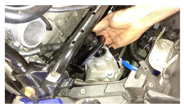
now you can push the engine mount bolts part way out so they are just flush with the engine mount bracket making room to slide the power steering mount plate into place on the engine mounts. once in place you can push the bolts back in and put the nuts on but don't tighten them yet.
