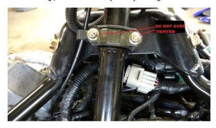
Once you have the bushing back together and snugged to the correct amount you can reinstall the handle bar riser back on to the post.
