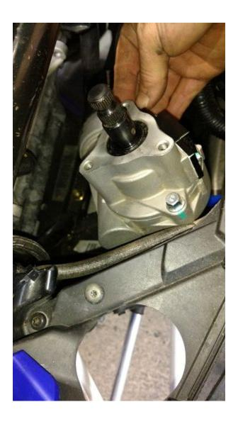
now you will need to put the power steering mount plate into place. you must get the mount plate down in near where it goes and then position the motor in just the right place so the plate will slide down over the shaft and into place. see picture on next page
