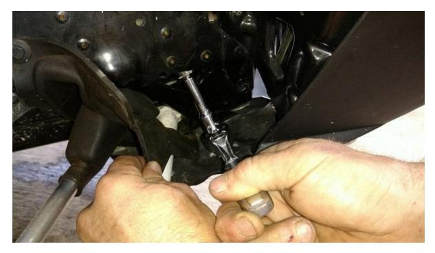
Next step is to remove the nut from the bottom of the steering post using a 17mm deep socket and ratchet.
