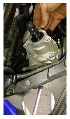
**Important:** When installing the set screw in the lower end of the steering post you will first want to look in the hole and make sure it is lined up with the groove in the steering motor shaft. Once you have it lined up you can put the set screw in and tighten it up with a 5/32 Allen wrench. Next be sure to tighten the jam nut using a ½ inch wrench.
