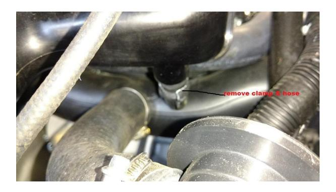
Next you can loosen the clamp on the blow off valve shown in the picture above and then pull the hose off and swing it off to the RH side.
