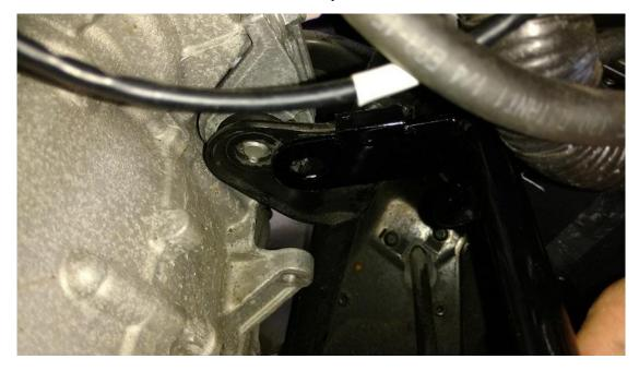
Once in place you can push both engine mount bolts back in all the way and put the nuts on the do not tighten them yet. Next you can install and tighten the three bolts in the steering motor. See picture below.
