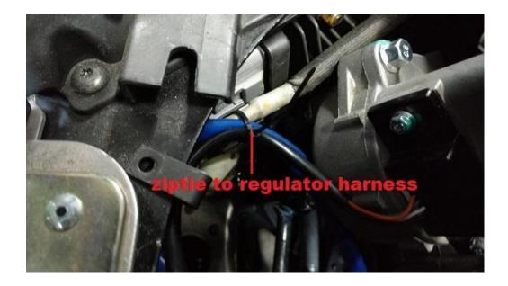
Now you can plug the power source harness into the module and route it and the single white wire up along the male harness of the snowmobile. See picture below.
