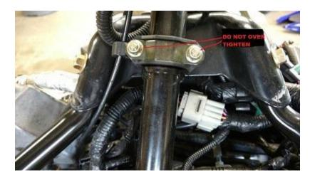
Next step is to install the power steering control module.
