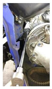
Next step is to remove the motor mount nuts. First remove the clutch side using a 15mm socket and a long extension on the bolt.
