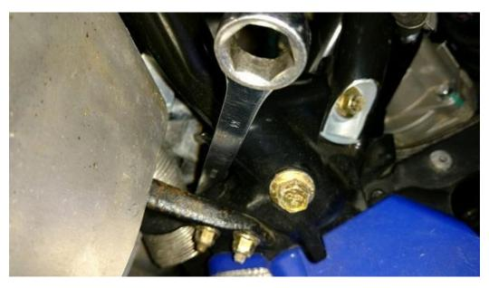
Once the exhaust side nut is off you can slide the bolt out part of the way so that it is just even with the bracket.
