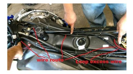
Connect white wire using the supplied red connector to the ted w/blue stripped wire from the accessory plug.
