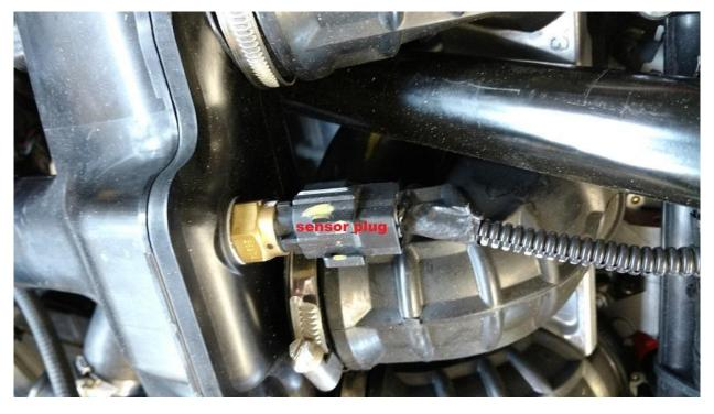
Next remove the hose from the lower RH side of the airbox shown below then remove the airbox.
