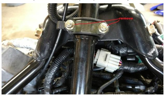
Next step is to remove the nuts from the upper steering post bushing using a 10mm socket. Once the nuts are removed you can take the top half of the bushing off.
