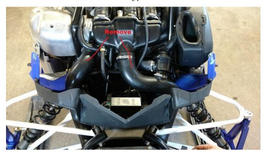
Next remove the small hose from the upper side of the airbox shown below.
