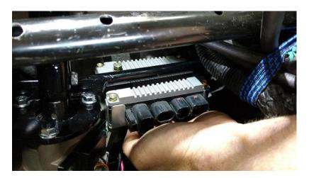
Snug the two bolts using a 10mm socket. Next you can plug the motor wires into the module. See picture below
