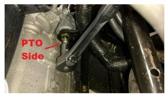
Once the nut is off you can slide the bolt part way out - leave it flush with the bracket. Now you can remove the other side motor mount nut using a 15mm open end wrench and the same 18mm socket. See below –
