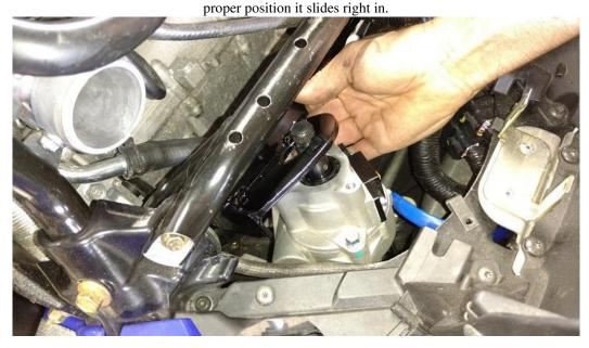
Once the mount plate is slid over the upper shaft you can slide the mount plate into position on the engine mounts. See below picture.
