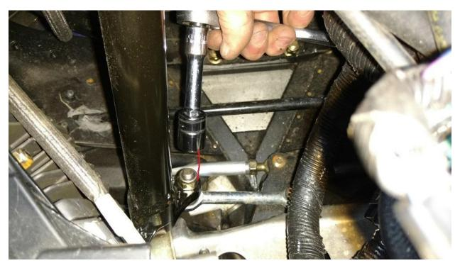
Next you will want to remove the nut from the steering link rod in the front of the bulkhead seen in the picture above.
