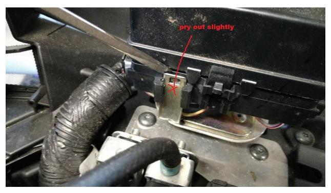
Next remove the fuse box by prying the holding tabs out and lifting on the fuse box, shown above. Then pull the fuse box off to RH side out of the way.
