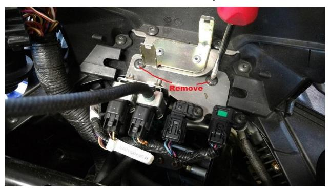
Next remove the screws from the sensor/ relay mounting plate picture next using a T25 torx driver. Also swing this plate to the RH side out of the way.
