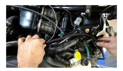
The white wire will branch off towards the clutch cover where you will see a single orange wire in which you will use the supplied red connector to connect to it.
