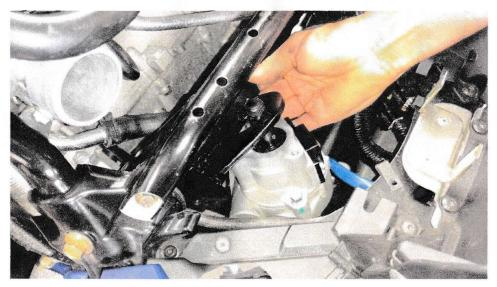
Now you can push the engine mount bolts part way out, so they are just flush with the engine mount bracket making room to slide the power steering mount plate into place on the engine mounts. Once in place you can push the bolts back in and put the nuts on but do not tighten them yet.
