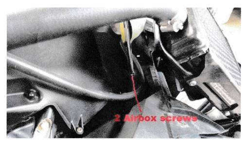
Once the lower airbox screws are removed you can loosen the three intake clamps and then prepare to pull the airbox out. You will need to unplug the sensor and pull the hoses and tube from the airbox, but the tube will need to be pulled out as you are removing the airbox.
