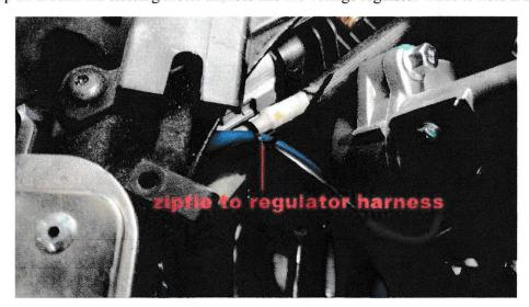
Next plug in the power supply wire harness and run it alone with the snowmobiles main wire harness up the clutch side all the way to the top. See picture below
