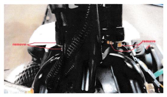
Next remove the bolts from the lower side of the handlebar riser. Picture above.
