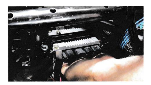
Next you can plug the motor wires into the module. See picture below
