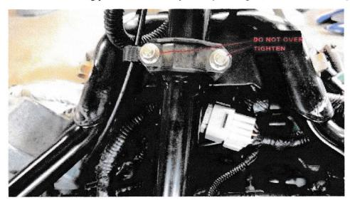
Once you have the bushing back together and snugged to the correct amount you can reinstall the handlebar riser back on to the post.
