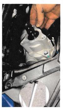
Now you will need to put the power steering mount plate into place. You must get the mount plate down in near where it goes and then position the motor in just the right place so the plate will slide down over the shaft and into place. See picture on next page
