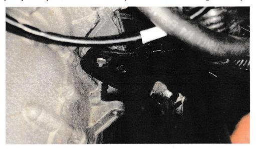
Next you will need to install the bolts in the power steering motor and tighten them using a 10mm socket and ratchet, see the picture on the next page
