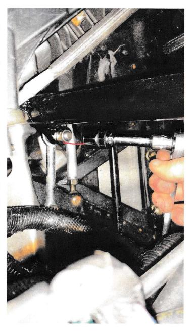
Next you will need to remove the 6 push darts in the RH rubber boot that covers the tie rod and suspension. See picture below
