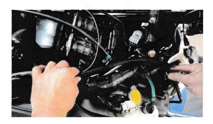
The white wire will run with the main steering harness up by the top of the gas tank and down the right-hand side to the accessory plug. We have included a splitter so you can still use your accessory plug for other items. Use the supplied blue connector on the end of the white wire and plug into the accessory splitter.
