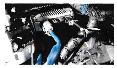
Put a zip tie around the steering motor harness and the voltage regulator wires to hold it in place.
