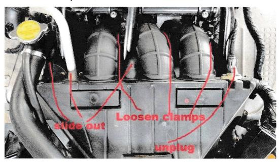
Once you have removed the airbox you can remove the lower handlebar clamp bolts. See picture on next page.
