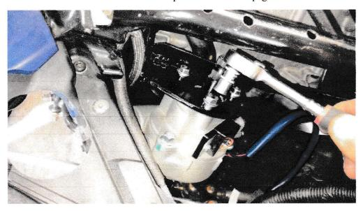
After you tighten the power steering motor mounting bolts you can go back and tighten the engine mount bolts.
